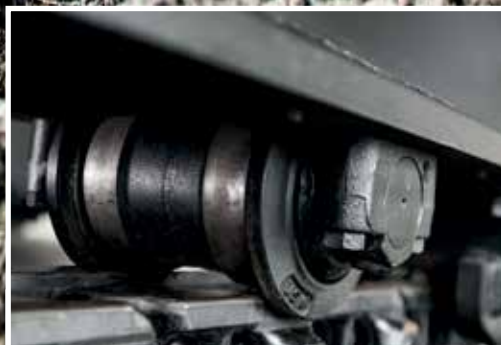
Strengthened bushing material improves wear resistance.
