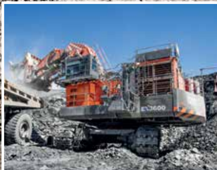
EX ultra-large excavators
