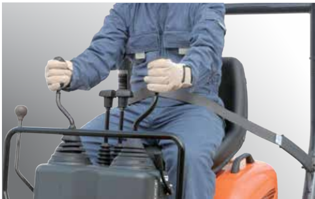
Hydraulic pilot control levers ensure a smooth operation.
