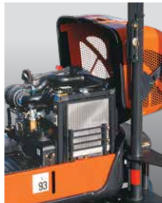
Wide-opening covers allow for easy maintenance.
