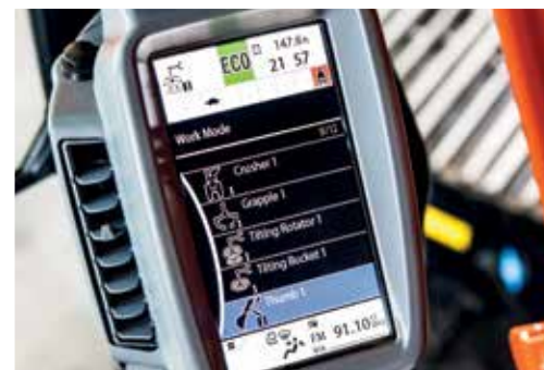
Two tilt modes add to the versatility of the ZX190W-6.
