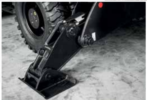
Reliability is enhanced by a reinforced outrigger cylinder cover.
