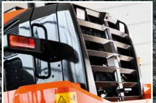
Optional anti-clogging radiators enhance durability.
