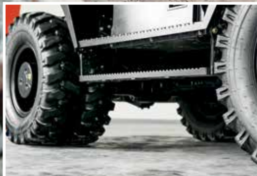
High ground clearance reduces damage from obstacles.
