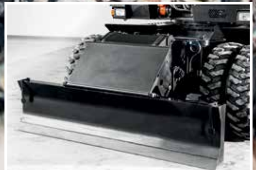
Large blade cylinder cover offers greater protection.
