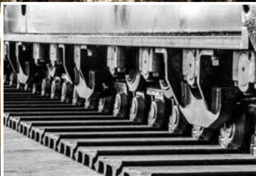
More track guards enhance the durability of the track link.
