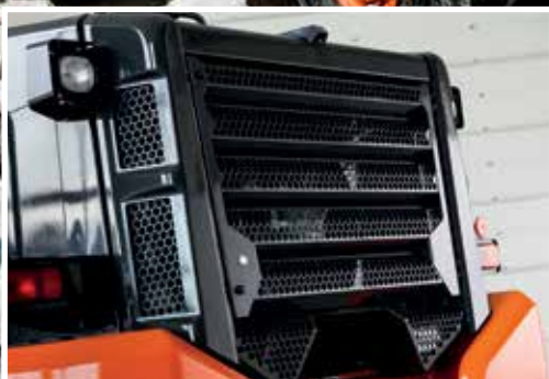
New rear grill protects radiator compartment.
